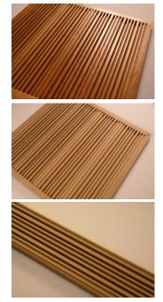
Using Manfred Schroeder's diffraction number theory, our new HighTones2 Diffuser design offers improved "equal energy" diffusion. This is accomplished via two design methods: a higher order well sequence, offering more available well depths for smoother diffusion; and Barker code implementation, offering reduced lobing that results from repeated sequencing (Fig. 2).
