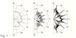
**Multiple Panels -** Multiple 11-well sequences are required for the QRD to achieve equal energy lobes (four or more are recommended). However, as the number of sequnces is increased, reinforcement leads to narrower and stronger lobes (Fig. 1). Incorporating a Barker code breaks up the modulus lobing (Fig. 2).
