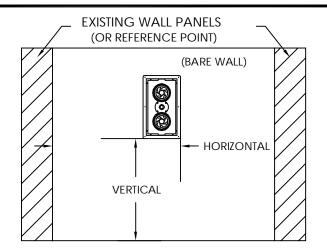
MEASURE SPEAKER ON THE WALL AND TRANSFER THESE DIMENSIONS TO THE BACK OF THE WALL PANEL.
