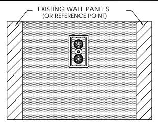
LOCATE WHERE PANEL NEEDS TO GO ON THE WALL AND DRY FIT OVER SPEAKER USING THE PROVIDED IMPALING CLIPS
